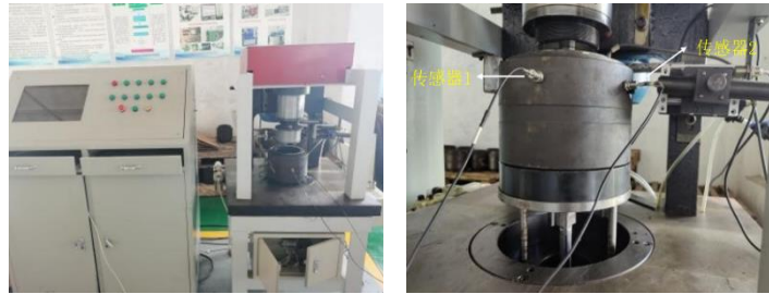
(a) Dynamic Performance Test Bench for Railway Bearings (b) Vibration Sensor Positions
