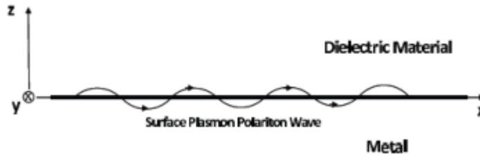
Figure 1. Surface Plasmon Polariton wave model
