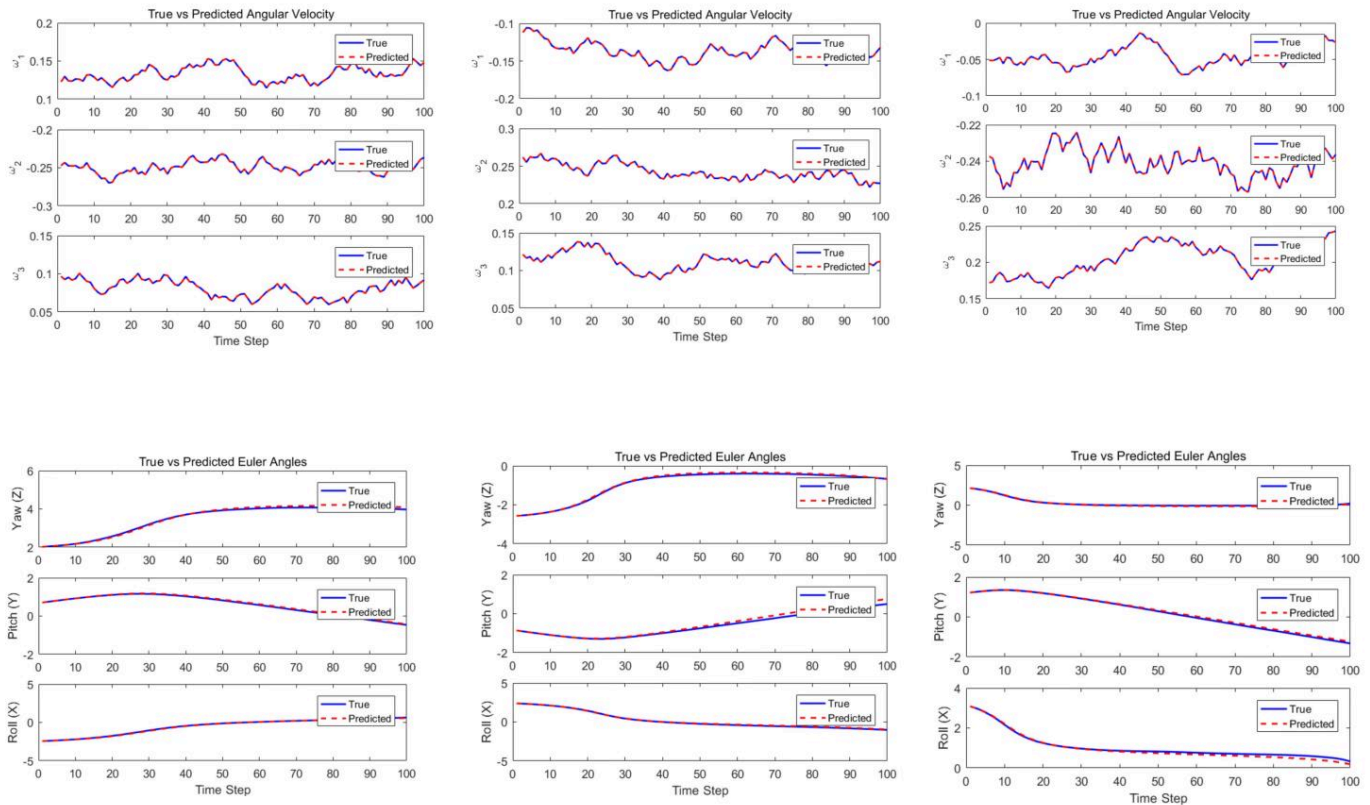
Figure 4. Prediction results of angular velocity and Euler angles for three representative test trajectories using the Koopman-based model
