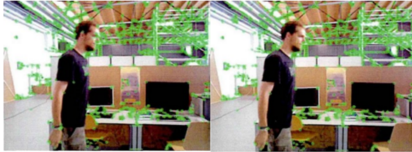
Figure 6. Results of dynamic point filtering based on dense optical flow
