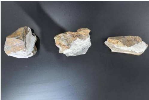
Figure 1. Condition of the stone block bonding surface
