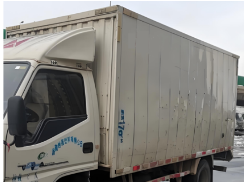
Figure 3. Deformation of the side panel
